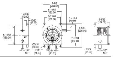
The popular Series AT22000 ATEX Approved Series 2000 Magnehelic® Differential Pressure Gage is now available in a flame-proof ATEX enclosure with the new ATEX approved AT22000 Series. This gage can indicate positive, negative or differential pressures and is accurate within 2%.
